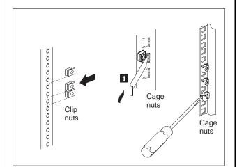
Using the attached template and stickers, mark the appropriate holes on your rack in the locations indicated by the arrows on the template. Install the clip nuts or cage nuts as required for your rack cabinet.
