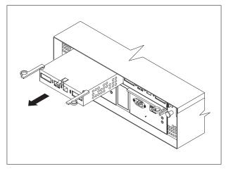
Remove the RAID controller by pushing down on the latch that is centered on the controller. Grasp the pull-rings on the levers and pull them to remove the RAID controller. Set it aside for later installation.
