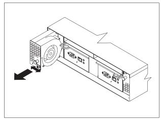
Remove the hot-swap fan by sliding the latch on the fan to unlock it. Pull the handle and remove the fan from the storage server.
