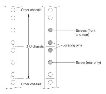
5. Install one thumb screw into the front rack-cabinet EIA rail as shown in the following illustration.
