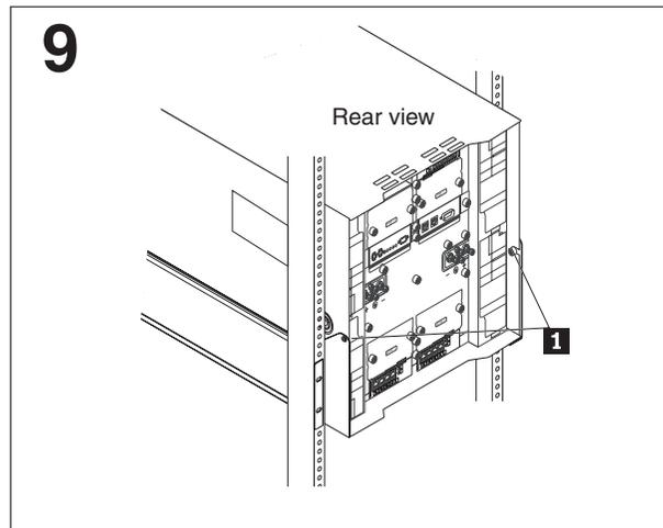
From the rear of the rack, secure the two captive screws, located in each blower bay, to the shelf brackets **1**. Reinstall the blowers in the BladeCenter T unit. (See the *BladeCenter T Types 8720 and 8730 Installation and User's Guide* for installation procedures.)
