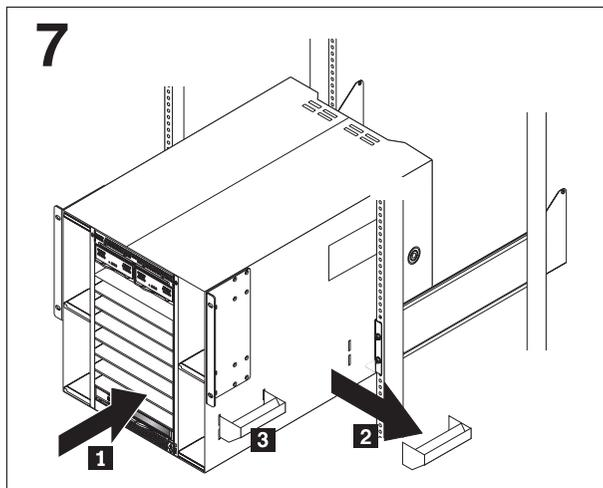
Carefully lift and place the rear edge of the unit on the front of the shelf brackets. Slide the unit along the shelf brackets until the rear lift handles are close to the front flanges **1**.
