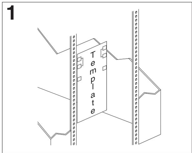
Position the template on the rack so that the edges of the template do not overlap any other devices to be installed. Line up and select the holes on the front and rear of the rack in the locations indicated by the arrows on the attached template.
