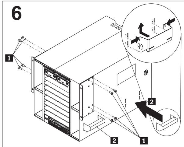
Attach the two mounting brackets to the sides of the unit by installing eight M4 flathead x 8mm screws **1**.
