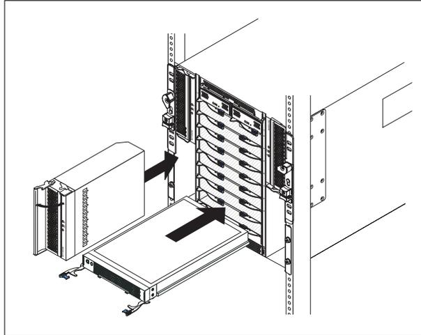
Carefully reinstall the power modules **1** , blade servers **3** , and bezel assembly in the BladeCenter T unit. (See the *BladeCenter T Types 8720 and 8730 Installation and User's Guide* for installation procedures.)
