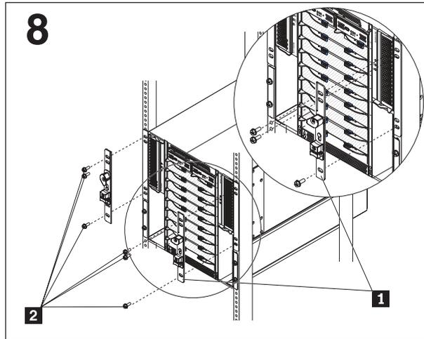
Align the holes in the bezel lock bracket **1** with the holes in the mounting bracket; then, secure the bezel lock and mounting bracket to the shelf bracket with three M6 combination-head screws **2**. Repeat this step on the opposite side.
