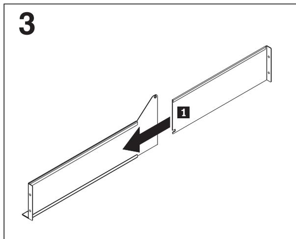
Assemble the shelf bracket by inserting the rear rack bracket into the shelf bracket **1**.
