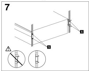
Press in on the slide-rail safety latches so that you can slide the server fully into the rack cabinet. Ensure that the rear slide-rail brackets are vertically aligned; then, fully tighten the rear M6 screws 1 on both slide rails.
