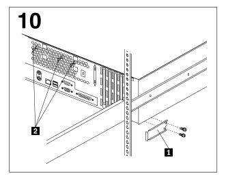
Use two M4 screws to install the cable-retainer bracket 1; then, install the cable clamps 2 in the second row of holes as shown.
