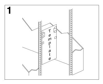
Use the attached stickers to mark the holes on the front and rear of the rack cabinet as indicated by the arrows on the attached rack mounting template.
