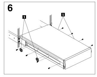
Use four M4 screws per side to secure the server to the rails; then, remove the rack-support wheels 1 and store them in a safe place.
