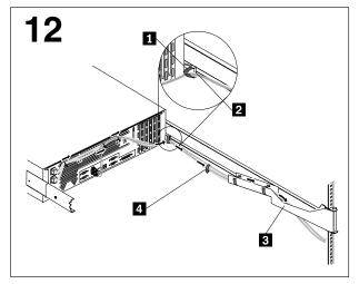
With the slide rails fully extended, attach the cables to the cable-retainer bracket 2. Determine the length of cable needed between the server and the cable-management arm; then, route the cables through the cable-management arm 3. Use cable straps to secure the cables to the bracket 1 and to each other 4.
