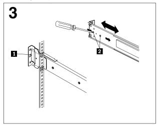
Use the tab 1 on the rear of the slide rail to align the slide rail to the rear of the rack cabinet. If it is necessary to adjust the length of the slide rail, loosen the screws 2 on the rear of the rail.
