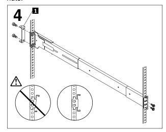
To install the left slide rail, ensure that the front slide-rail brackets are vertically aligned; then, insert and fully tighten both front M6 screws. Install the hinge bracket 1 before you insert the rear screws; then, partially tighten both rear M6 screws.
