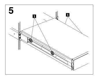
If you loosened the screws to adjust the length of the rail, tighten them now; then, fully extend the slide rails out of the rack cabinet until the slide rails lock into place.
