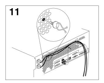
Attach the power, keyboard, mouse, and monitor cables (if required) to the rear of the server. Route the cables through the cable clamps; then, attach all other required cables to the server.
