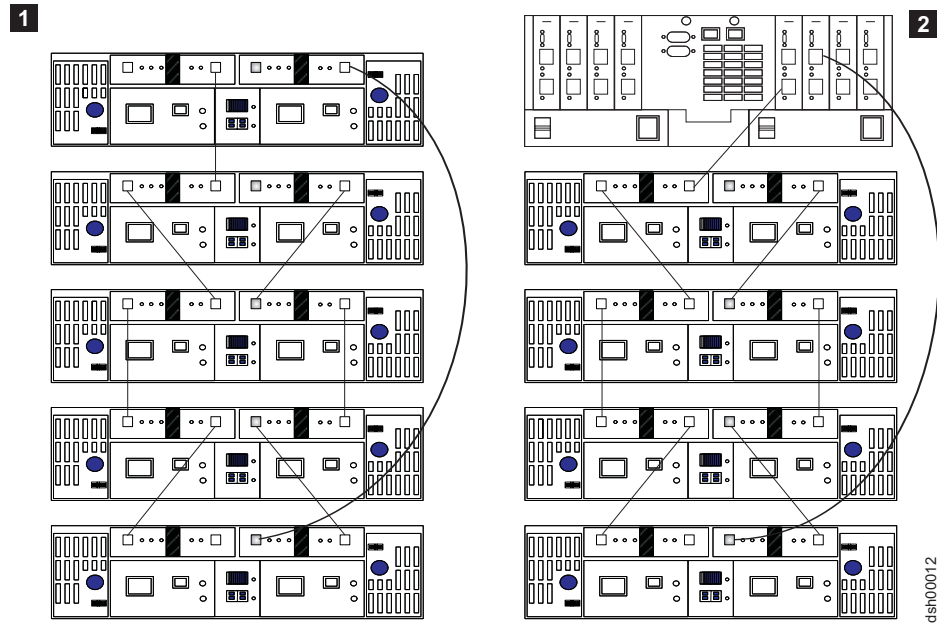
Figure 12. Alternate cable loop schemes possible but not recommended when connecting DS4000 storage subsystems (4 of 4)
