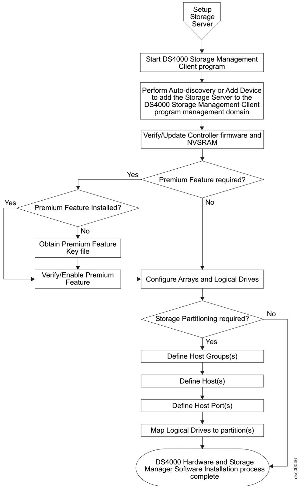
Figure 10. Installation process (part 6 of 6)
