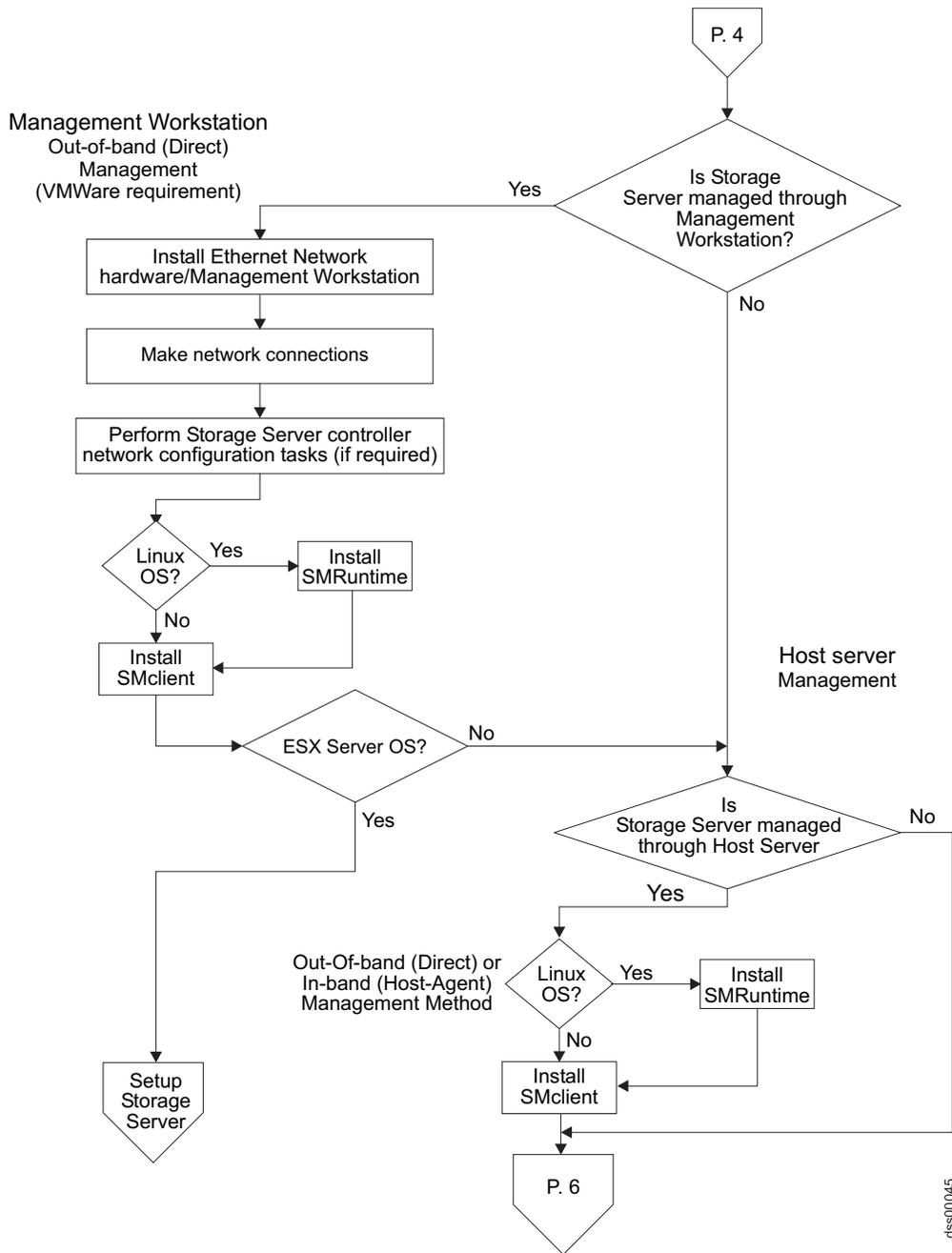
Figure 8. Installation process (part 4 of 6)
