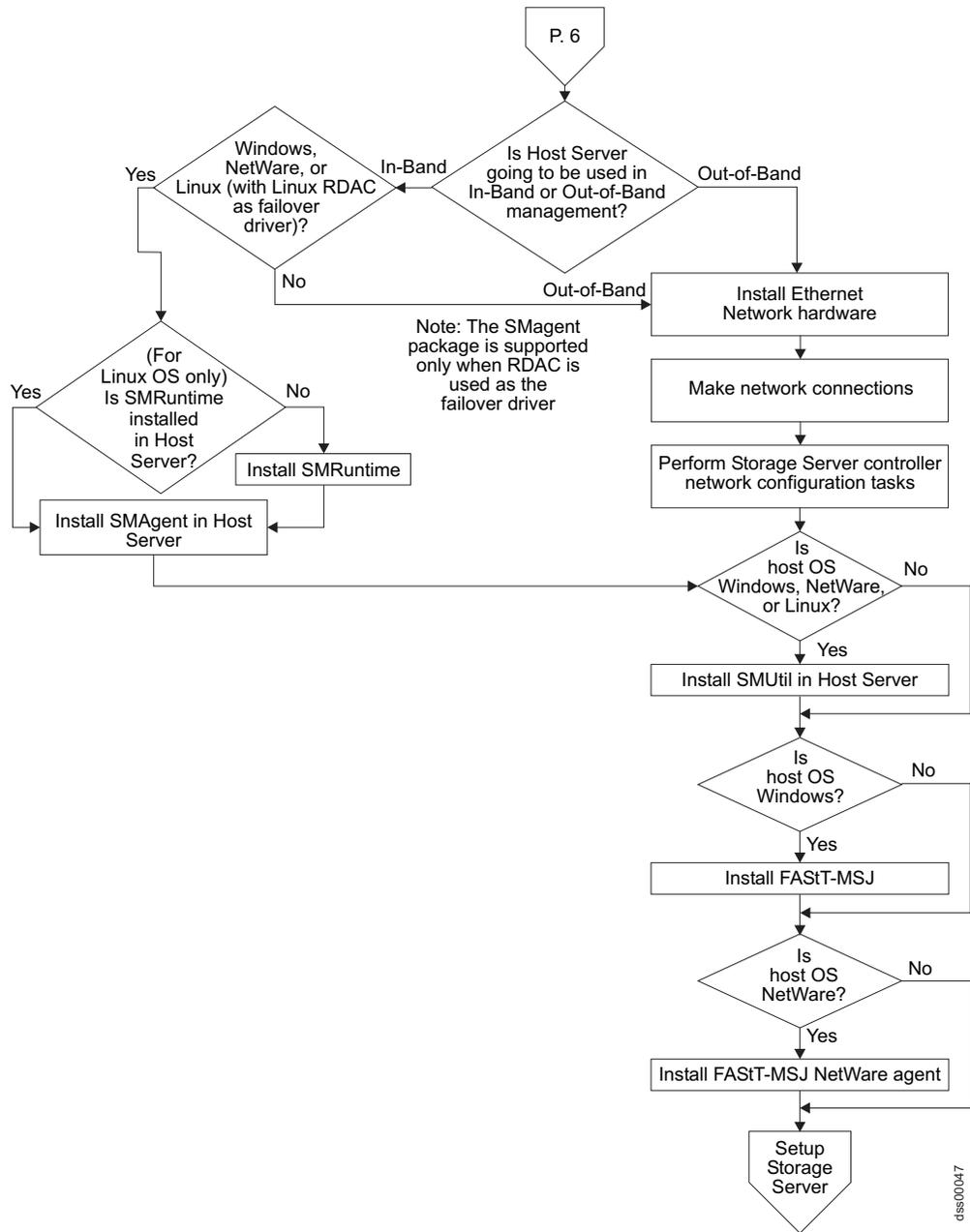
Figure 9. Installation process (part 5 of 6)
