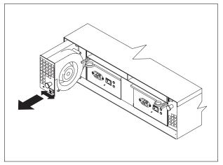
Remove the hot-swap fan by sliding the latch on the fan away from the center of the unit to unlock it. Pull the handle and remove the fan from the storage server.
