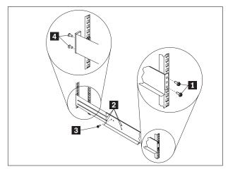
On the rail marked **R**, remove the 6-32 in. screw and loosen the four screws **2**. Hold the front of the rail against the outside of the right rack-mounting-flange and loosely install two M6 screws **1**.
