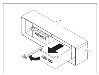
Remove the power supply by grasping the pull-ring on the power supply lever and squeezing it to release. Pull the lever fully open and remove the power supply from the storage server.
