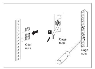
Using the attached template and stickers, mark the appropriate holes on your rack in the locations indicated by the arrows on the template. Install the clip nuts or cage nuts as required for your rack cabinet.
