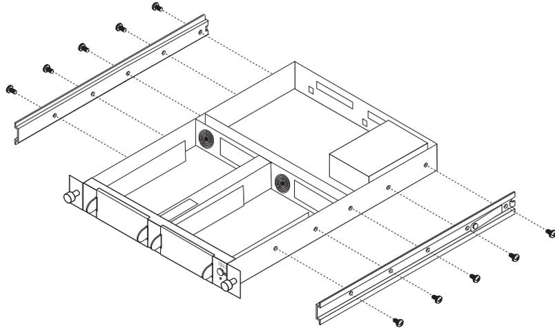
4. Attach the rear-rack rails to the front-rack rails. (The four 10-32 x 1/2-inch screws and nuts are provided in the miscellaneous hardware bag.)
