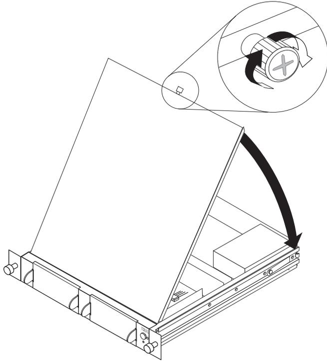
9. Install the tape enclosure in the rack:
