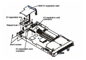
Figure 5. -JS20 Blade FC Expansion card layout
