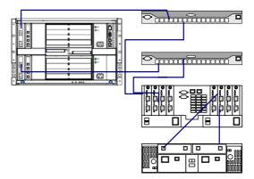
Figure 2.- BladeCenter in Fabric-attach SAN environment
