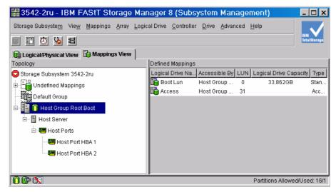
Figure 9. - DS4000 series Host-port mapping
