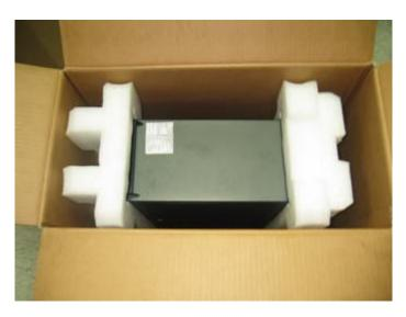
2.10 Place keyboard carton between the end of the carton and the rear of the PC. If no keyboard is called out use empty carton 25P1068.
