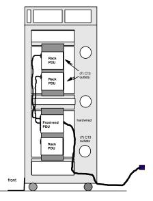
One other very nice feature of the Enterprise Rack is the fact that it has 4 1U pockets that are accessible and visible from the rear of the rack. It is possible with the Enterprise Rack to install a pair of PDUs in these 1U pockets using the horizontal mounting hardware.
