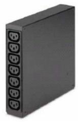
This PDU provides an economical, basic power distribution capability for rack-based systems, enabling you to satisfy the power requirements of each device without overtaxing your power source. It has one universal-voltage power input and supports up to seven devices with a combined power requirement of 1500W at 100Vac to 3600W at 240Vac (based on AC input volts).
