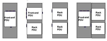
The illustration below further clarifies how the rack looks once these PDUs are installed. This example shows only a single "nest" but this could easily contain more than one per pocket.
