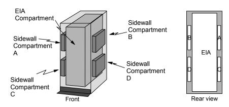
The depth of these side pockets allows the PDUs to be nested side by side for support of very large numbers of PDUs or KVM switches in the rack's pockets. Here are a few examples of the supported installations for the Enterprise Rack.
