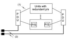
The last three topologies go a long way in preventing the majority of power problems that effect equipment today. All these topologies involve the use of a UPS product to add power conditioning and battery backup in case of an outage. Notice how much better the load on these PDUs is protected when used in combination with the proper UPS.
