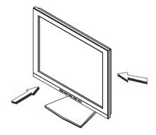
Before using your monitor for the first time, remove the clear protective film from the front of the screen.
