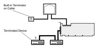
The following example shows SCSI devices connected to the internal connector.
