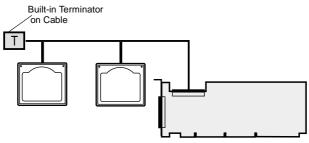
The following example shows SCSI devices connected to the external connector.
