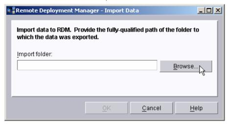
9. Navigate to the SCSITask folder, select the SCSITask.xml file, and select the OK button.
