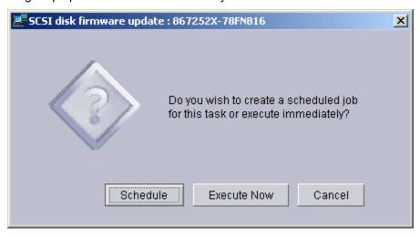
33. Click the **Execute now** button. The target system will wake up (i.e., automatically power itself on) and do a network boot.
