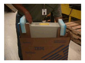
NOTE: When lifting the cushioned unit into the box, wrap arms fully around the cushions, and / use handle. DO NOT pick up the unit by partially grabbing the cushions or by lifting the cushions by the vent holes, other cavities, or ribs.
