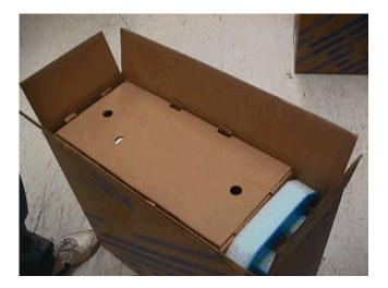
2.15 - Bend the top four flaps of the CPU carton inward (minor flap inside major flaps) so the scores are broken. Send the assembly down the conveyor to be sealed using IBM logo tape (74F5699 or 74F5698).
