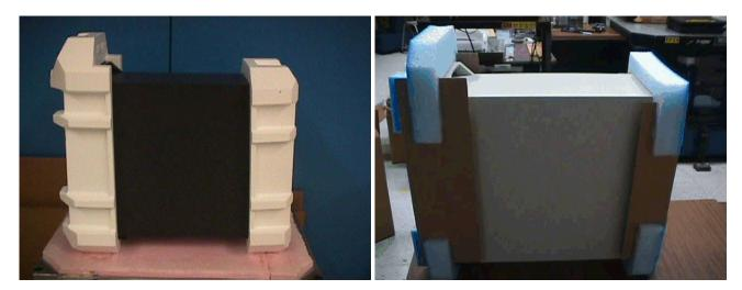
2.11 - Place the cushioned unit into the bottom of the carton.
