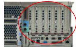
With four I/O buses, the x445 adapter slots will support two 133 MHz cards (each slot with its own bus), two 100 MHz cards (these slots share a bus), and two 66 MHz cards (these slots also share a bus). From the rear, the slots are oriented in order of ascending speed from left to right. Important Notes: 1) All slots support 3.3V adapters only and 2) because of the system depth, the blue handle must be removed when installing full-length PCI adapters.
