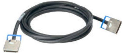
Along with these cables, there is also a corresponding 3.5-meter Interconnect Management Cable used to connect the RXE Management Port on the x445 to the RXE Management Port on the RXE-100. This cable (Option part# 31P6087) is also required for connecting multiple x445 systems together to ensure that the Service Processor is able to configure the systems under a single OS image.
