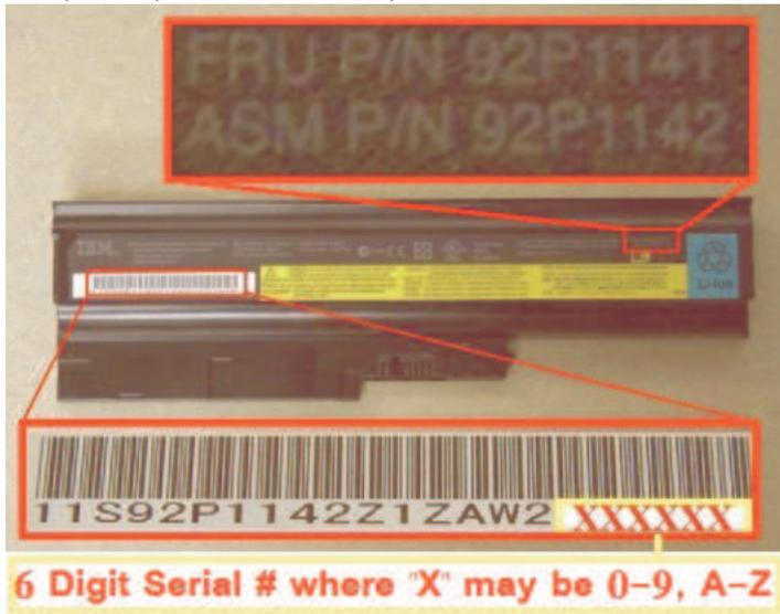
X60 and X60s 2.6 Ah, 4 Cell. Subs to FRU 93P5028 that is also recalled.
