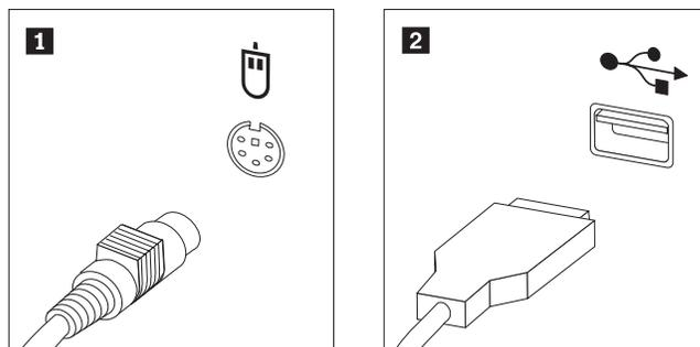
4. Disconnect the failing mouse cable from the computer.
