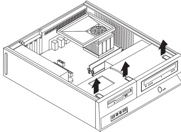
3. Slide the drive bay assembly forward until the drive bay assembly is aligned with the two slots on the sides of the chassis and remove the drive cables from the system board. Then pull upward on the handle **1** on the drive bay assembly to remove it completely from the computer.
