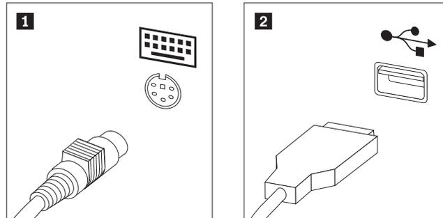
4. Disconnect the failing keyboard cable from the computer.
