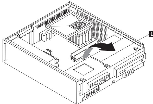
4. Disconnect the signal and power cables from the rear of the hard disk drive.
