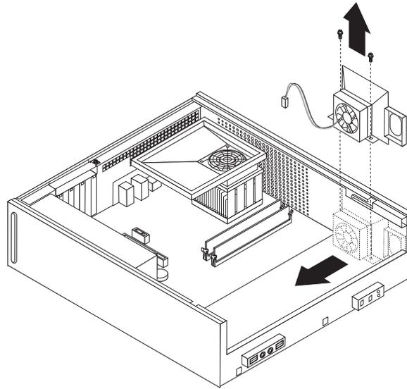
8. Install the new system fan assembly and install the two screws that secure the fan assembly.
