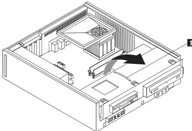
4. Disconnect the system fan cable from the system board. See “Identifying parts on the system board” on page 4.
