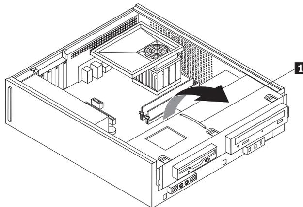
4. Release the optical drive by pressing inward on the blue retainer at the side of the drive.
