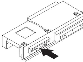
8. Align the drive bay assembly with the two slots and rails on the sides of the chassis, reconnect the drive cables on the system board, and then slide the drive bay assembly towards the rear of the chassis until it snaps into position.
