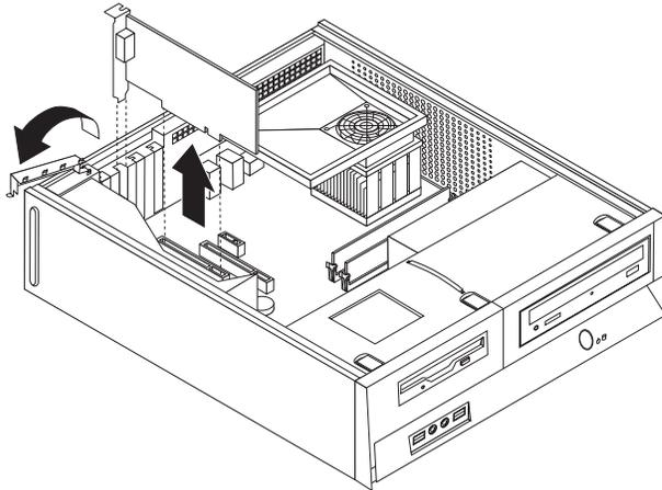
3. Remove the new adapter from its static-protective package.
