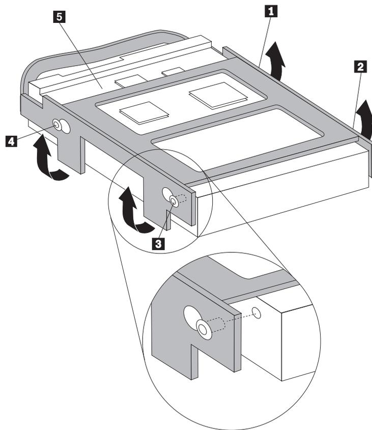
7. Position the hard disk drive and bracket so that it engages the retaining clips in the bottom of the chassis when you slide the bracket to the right.
