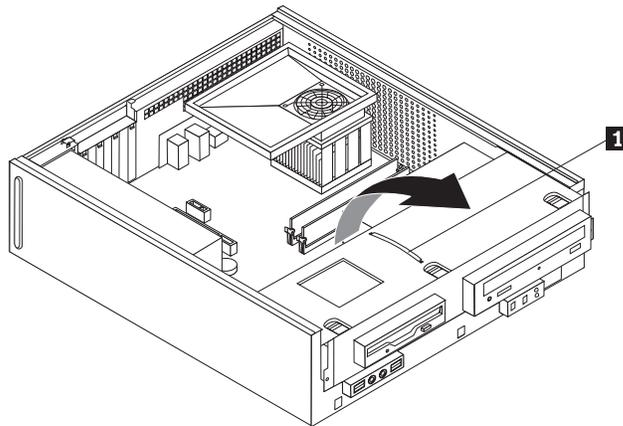
4. Release the diskette drive by pressing inward on the blue retainer at the side of the drive.
