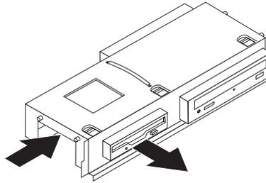
6. Remove the retainer bracket from the failing drive and install it on the new drive.
