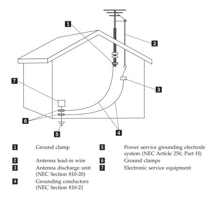
Figure 1. Proper grounding for the cable
