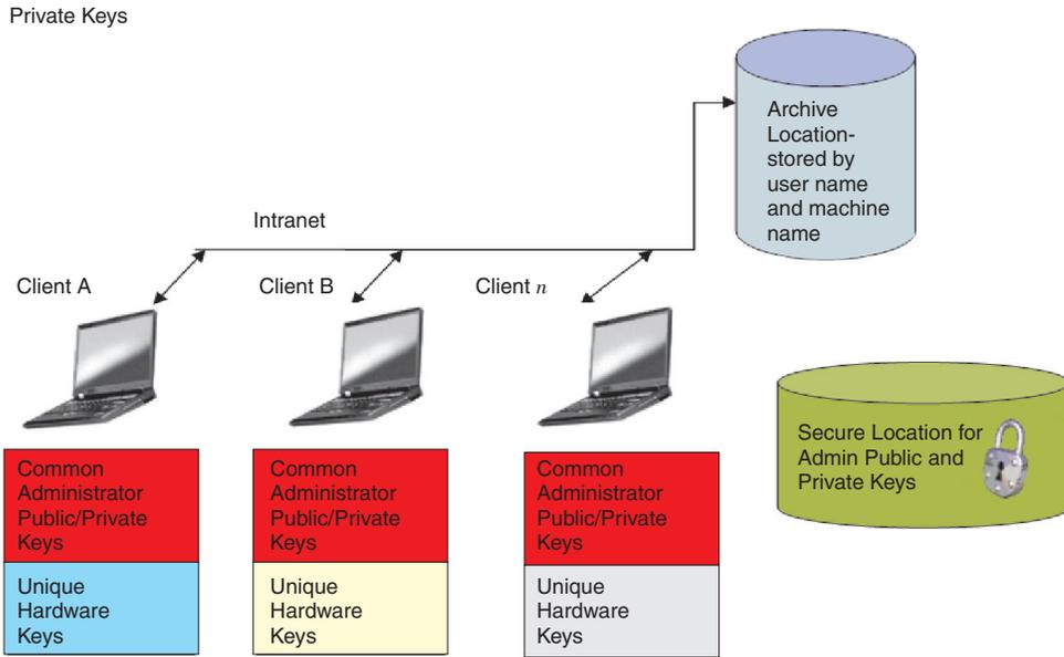
Figure 16. Major components of the IBM Client Security System.
