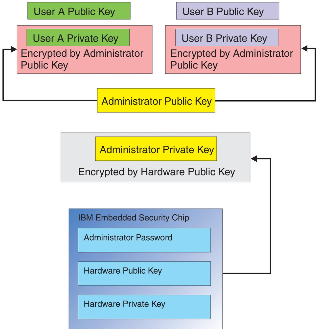
Figure 3. Several layers of encryption provide strong security
